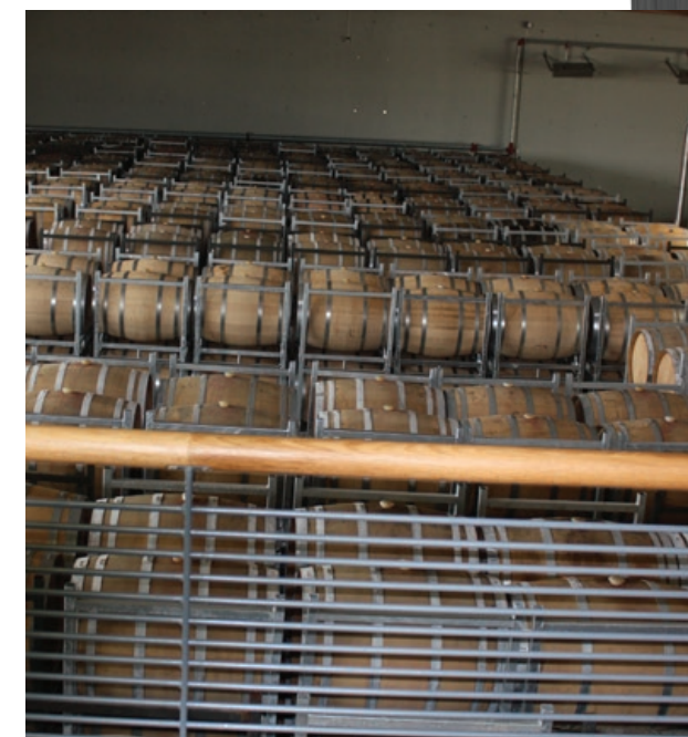
Barkan's barrel room, holding 5,000 oak barrels of aging wine, is the largest in Israel. The room must be kept at precisely 64.4°F at all times, and the barrels must be topped off every few weeks due to evaporation. A special misting system maintains high humidity.
